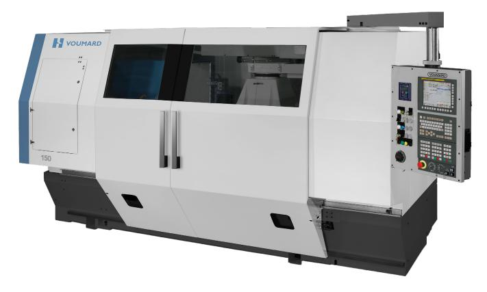
The VOUMARD VM 150 is a multi-purpose tool for ID/OD grinding operations with medium to large sized work pieces in small batches as well as in volume production. While short work pieces can be ground directly when clamped in the chuck, a variety of manual and automatic steady rests is available for grinding operations with long shafts.
